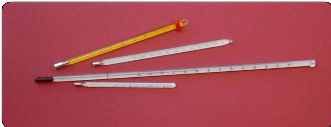
*Alcohol in glass and mercury in glass thermometers*
