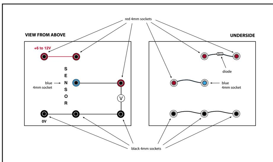
Temperature sensing unit construction
