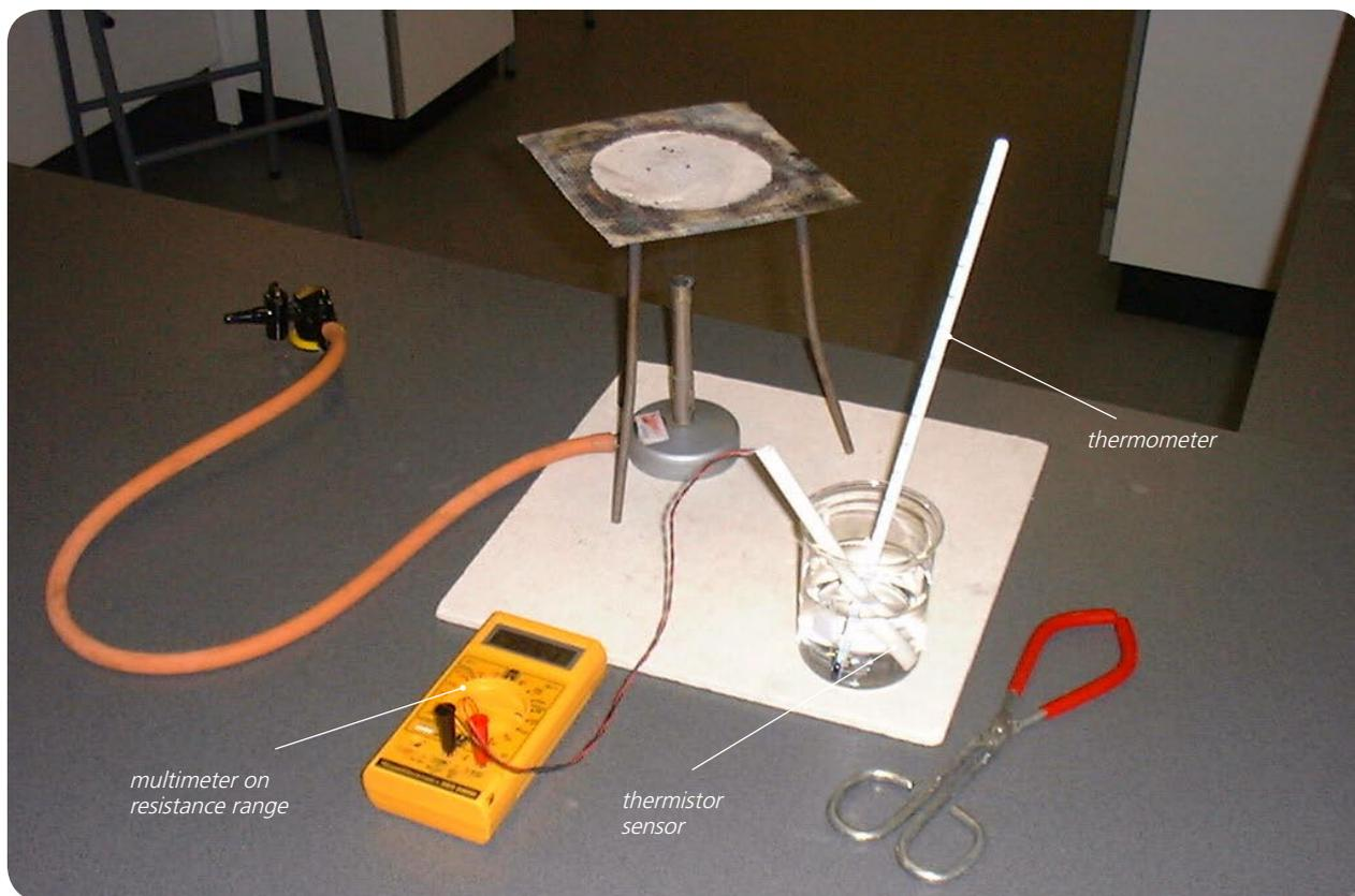
Set up of apparatus to measure the resistance of the thermistor at various temperatures
