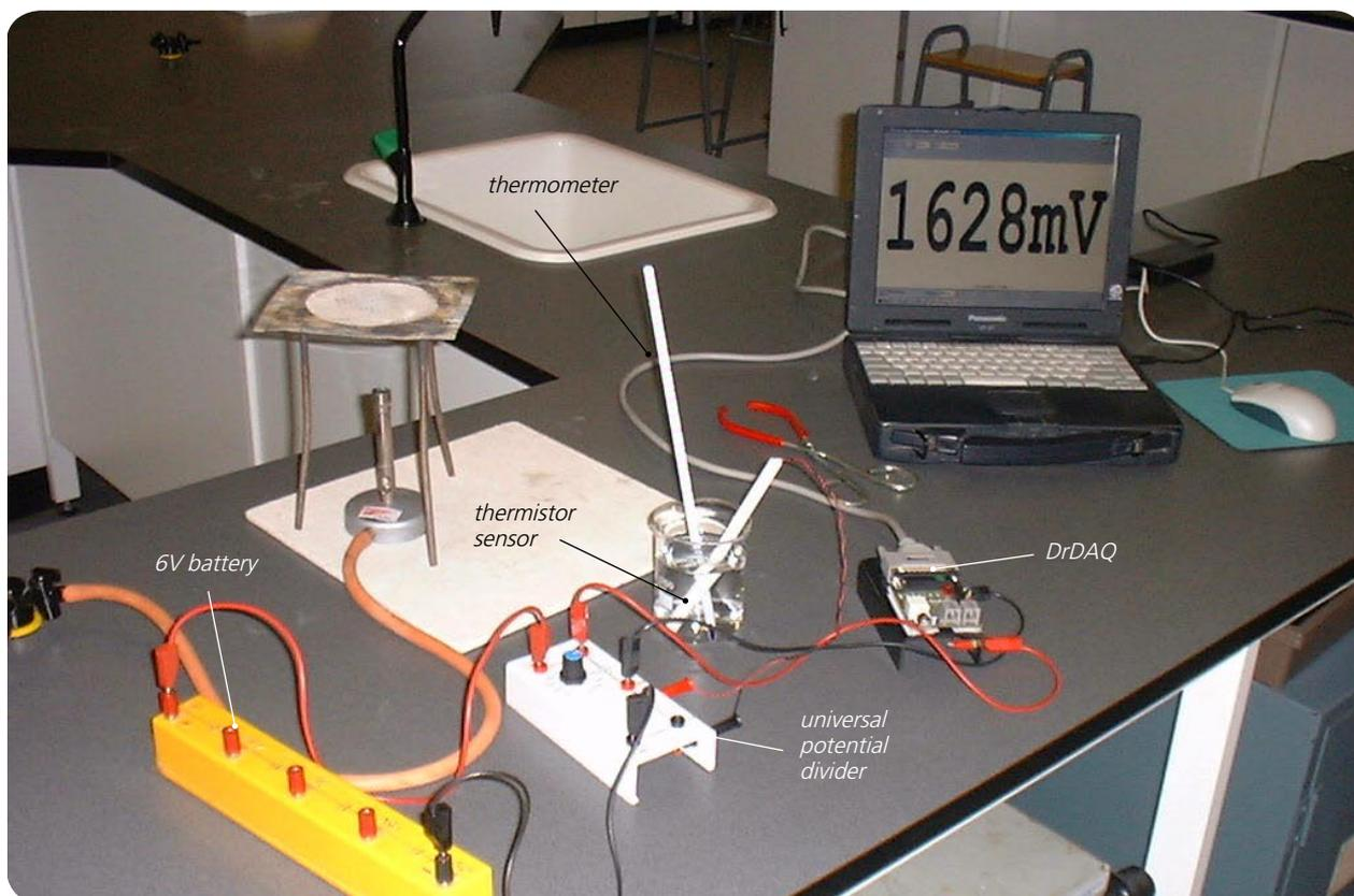
Set up of apparatus to measure temperature with a potential divider network, a thermistor and DrDAQ
