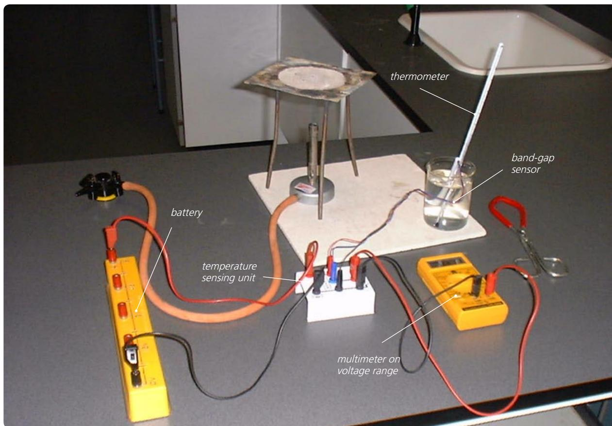
The LM35DZ connected to a multimeter
