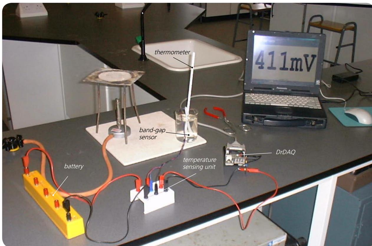
*Band-gap temperature sensor set up to use with PicoScope on DrDAQ*
