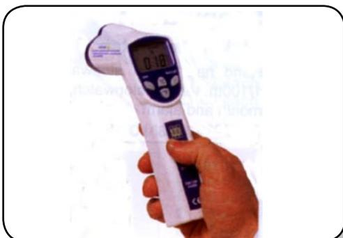
Laser pointing Infrared thermometer
