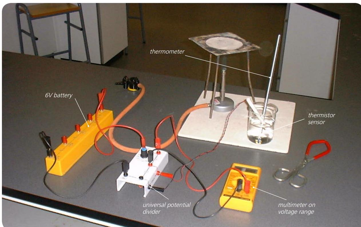
*Thermistor set up in a potential divider network*
