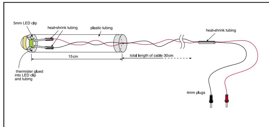
*Thermistor sensor construction*
