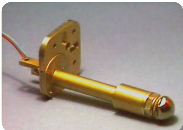
Piezoelectric force sensor on the Huygens probe (Courtesy Planetary and Space Sciences Research Institute, The Open University)
