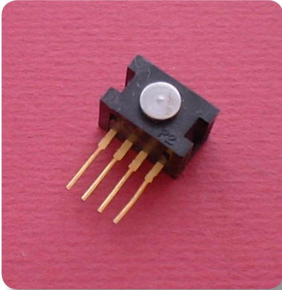
*Piezoresistive strain gauge*
