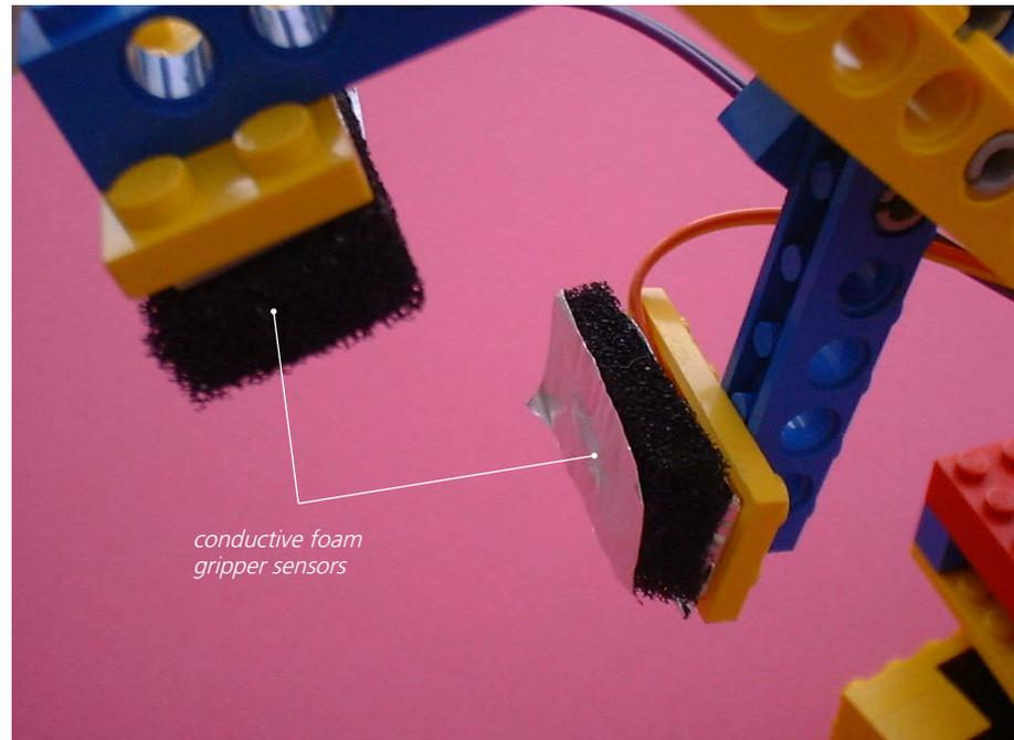
*Conductive foam gripper/bumper sensor*
