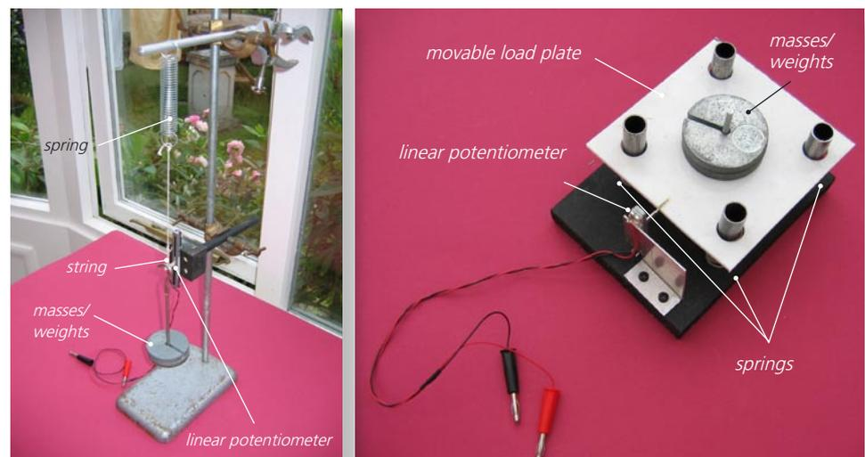
*Two sensors based on the movement of a linear potentiometer*
