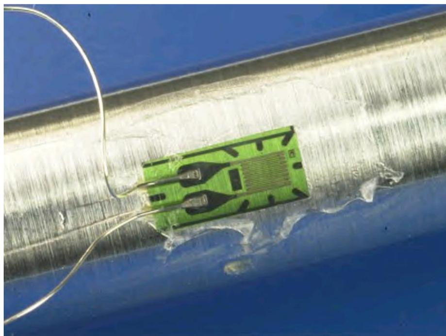
*Metal foil strain gauge (courtesy of DoITPOMS, University of Cambridge©)*
