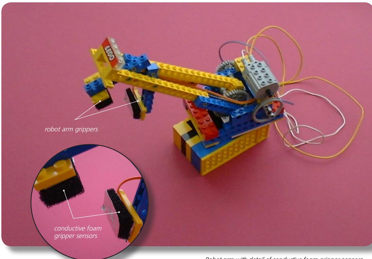
*Robot arm with detail of conductive foam gripper sensors*
