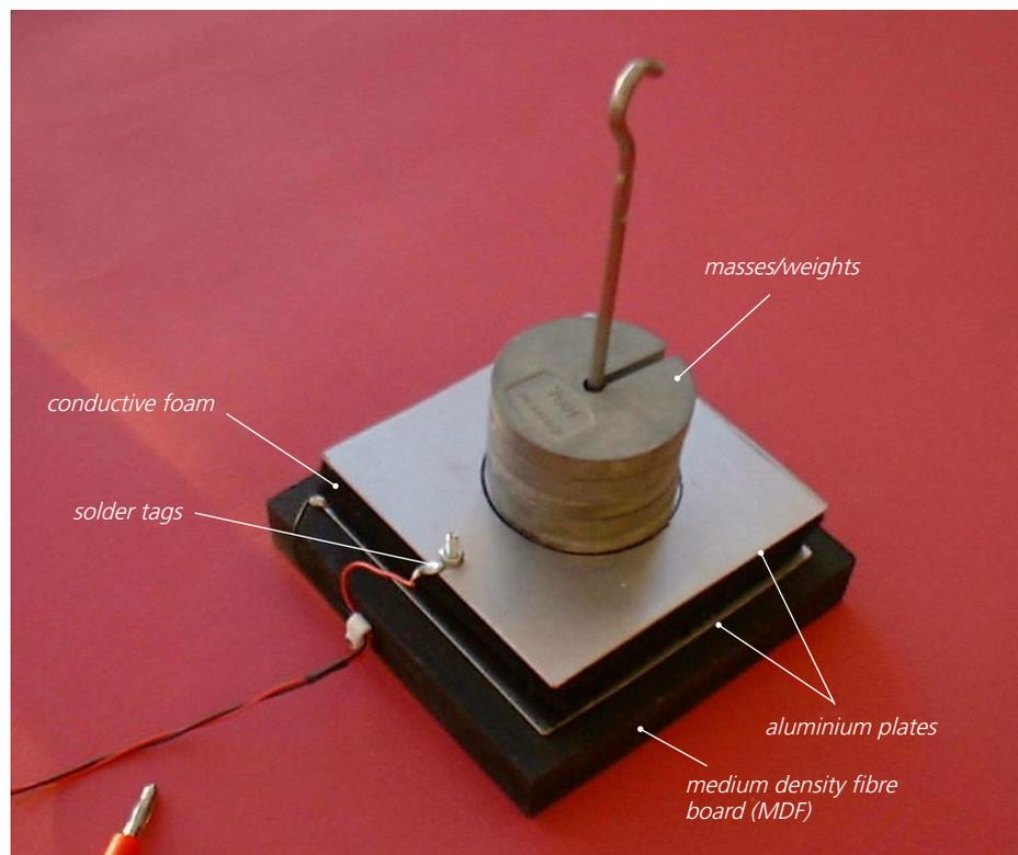
Construction of conductive foam sensor
