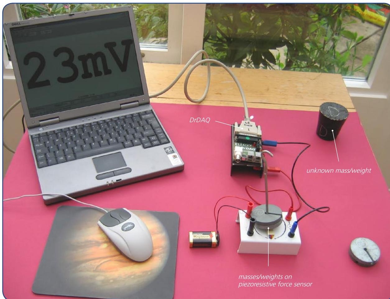
*Piezoresistive force sensor set up to use with PicoScope on DrDAQ*
