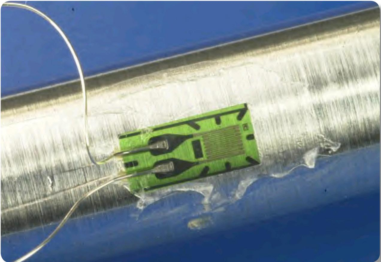
*Metal foil strain gauge (courtesy of DoITPOMS, University of Cambridge©)*
