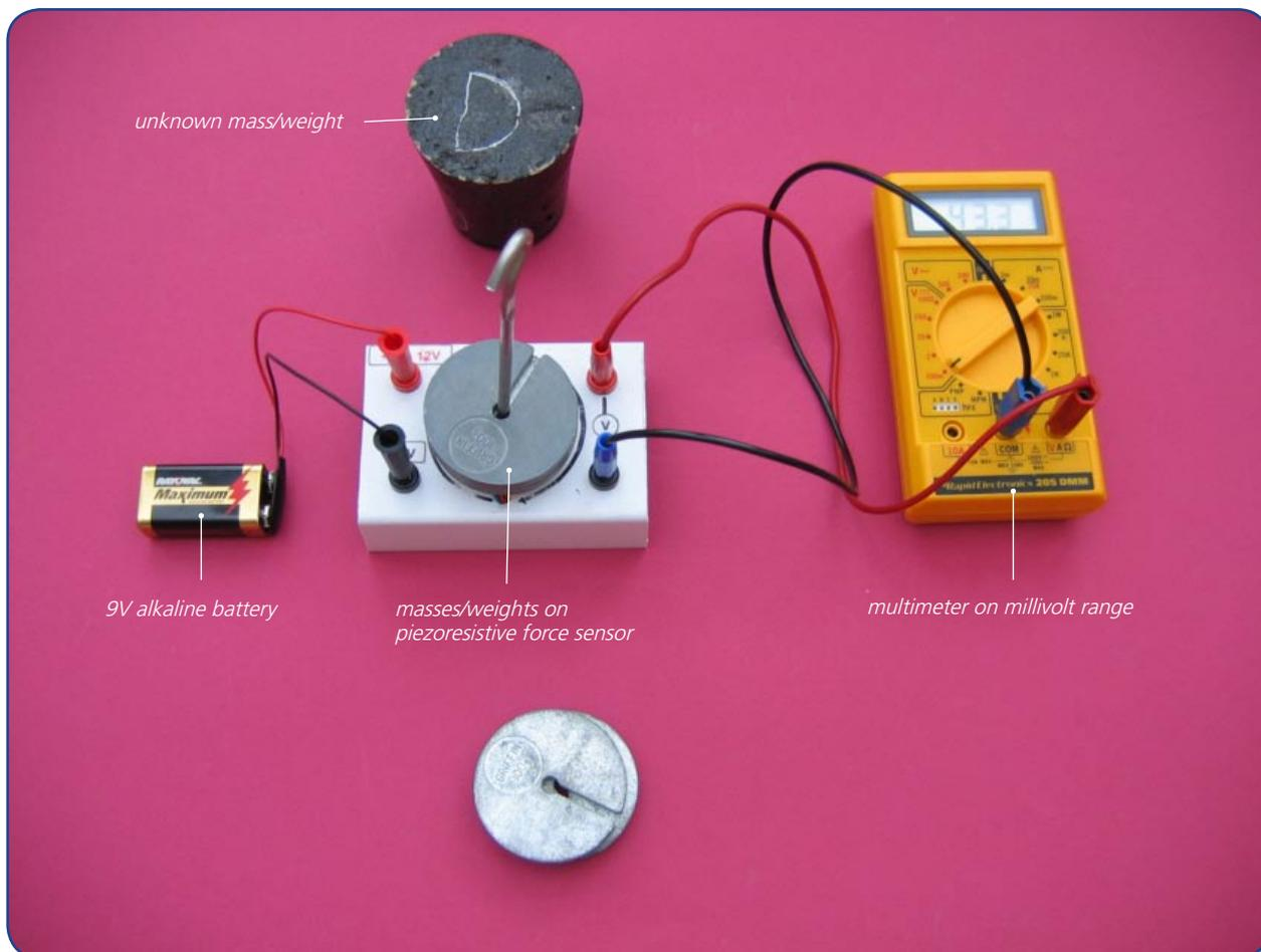
*Piezoresistive force sensor with output linked to a multimeter/millivoltmeter*
