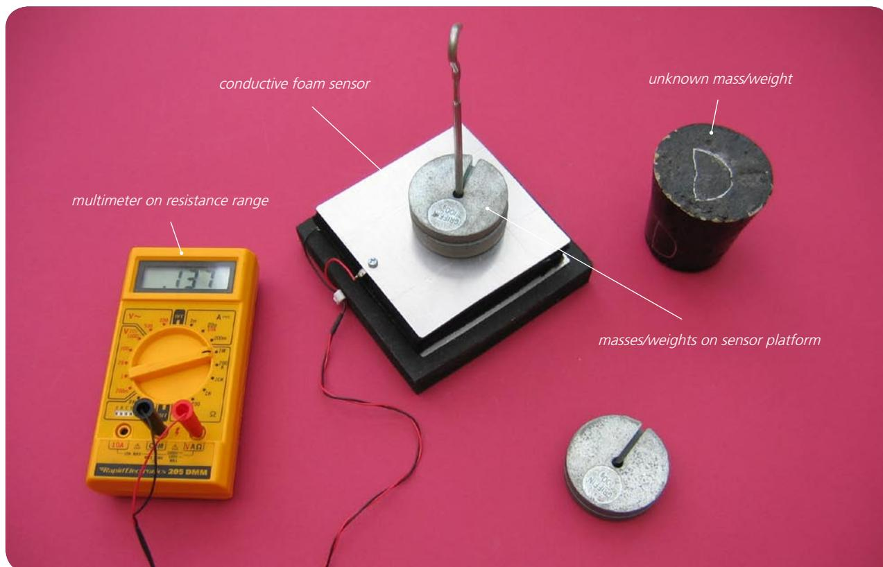
Conductive foam sensor connected to a multimeter on a resistance range
