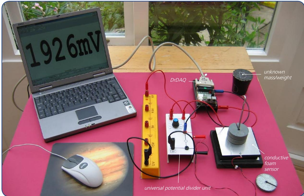
Conductive foam force sensor set up with a potential divider to use with PicoScope on *DrDAQ*
