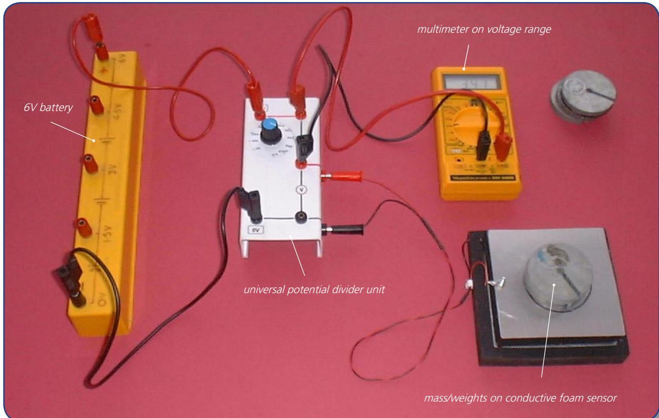
Conductive foam sensor set up for use in a potential divider network
